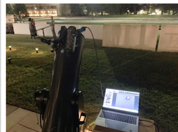
Ben's setup at the Archives. Scope points to Orion Nebula then people can view same object via astrovideo camera attached to a side mounted telescope. Best of both worlds!
